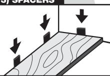
Designed for use against the wall to provide even expansion spacing
