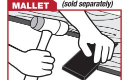
**Mallet provides efficient installation**
